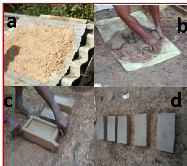
Fig. 2. a: Step 1: SDE Drying, b: Step 2: Mixing SDE with Clay, c: Step 3: Moulding, d: Step 4: Drying
