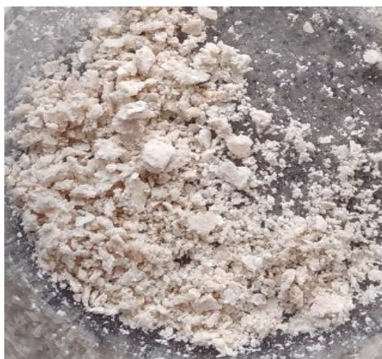
Fig. 1: Composite nanocellulose bio-adsorbent which was prepared using both rice husk and pineapple leaves
